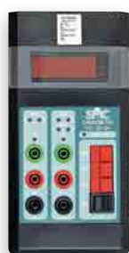
SMC PTE-30-CH Portable Relay Trip Timer
